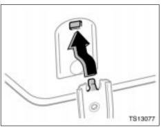
When the bottom cushion is reinstalled, click the claw of the hinge into the hole of the bottom cushion before refastening the dial.
