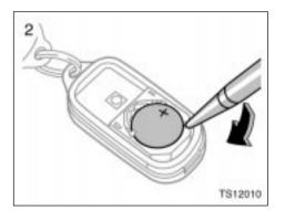
2. Remove the discharged transmitter battery by ballpoint pen.
