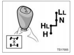
Use the four-wheel drive control lever to select the following transfer modes.
