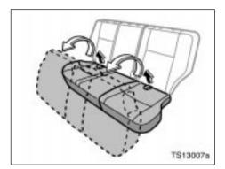
2. Swing the bottom cushion up by pulling the lock release strap.
