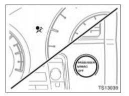
The SRS warning light will come on and front passenger occupant classification indicator light will indicate "OFF" if there is a malfunction in the front passenger occupant classification system. Contact your Toyota dealer as soon as possible.
