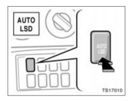
To turn on the system, push the "AUTO LSD" switch when the vehicle is stopped.
