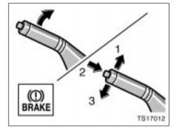
When parking, firmly apply the parking brake to avoid inadvertent creeping.
