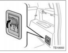
This power outlet is designed for use as a power supply for electric appliances.
