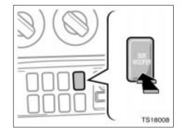
To operate the sub woofer, push the sub woofer on-off switch.
