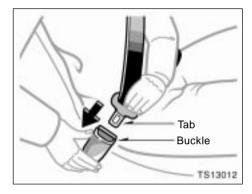
Adjust the seat as needed and sit up straight and well back in the seat. To fasten your belt, pull it out of the retractor and insert the tab into the buckle.
