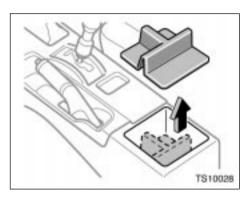
Type C cup holders are equipped with a detachable mat.
