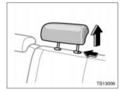
1. Remove the head restraint.
