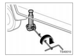
7. After making sure that no one is in the vehicle, raise it high enough so that the spare tire can be installed.
