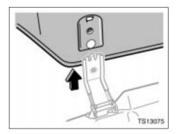
3. Separate the bottom cushion from the hinge.
