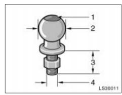
1 Trailer ball load rating 2 Ball diameter 3 Shank length
