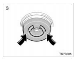
3. Install the rubber cover as shown and fit it securely on the boss. Plug in the connector.
