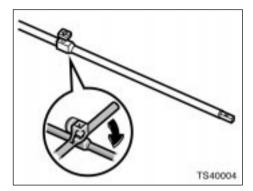
When connecting the jack handle extension(s) and jack handle end, use the jack handle to tighten the square head bolt. Make sure that the bolt fits into the depression on the joint.
