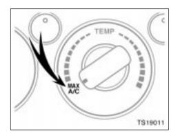
For quick cooling, turning the temperature selector knob fully towards COLD (MAX A/C) changes the air intake selector mode to RECIRCULATE.
