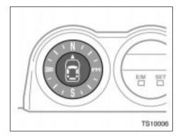
The compass indicates the direction that the vehicle is heading. In the above case, it indicates that the vehicle is heading north.
