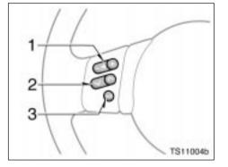
Some parts of the audio system can be adjusted using the switches on the steering wheel.
