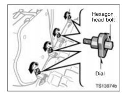
2. Loosen the bolts with the wrench at first and turn the dials with hands to remove them.
