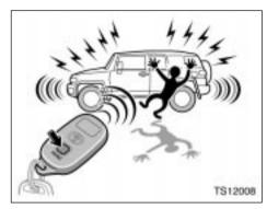
The "PANIC" mode does not work when the ignition key is in the "ON" position. This alarm function can be disabled. For details, contact your Toyota dealer.
