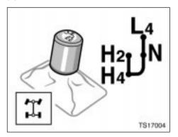
"L4" (low speed position, four-wheel drive): Lever at "L4"
