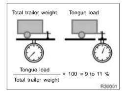
The trailer cargo load should be distributed so that the tongue load is 9 to 11% of the total trailer weight, not exceeding the maximum load of the following.
