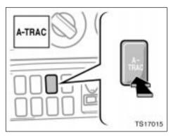
To activate the system, push the active traction control switch and shift the four-wheel drive control lever into "L4" (part-time four-wheel drive models) or "LL" (full-time four-wheel drive models). At this time, the active traction control system indicator light will come on.
