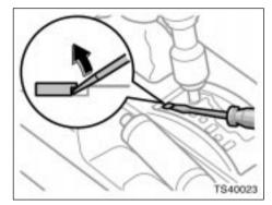
If you cannot shift the selector lever out of the "P" position to other positions even though the brake pedal is depressed, use the shift lock override button as follows:
