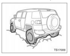
The rear differential lock system is provided for use only when wheel spinning occurs in a ditch or on a slippery or ragged surface.
