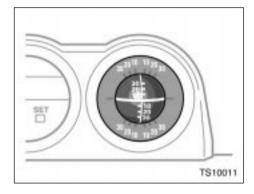
The clinometer shows longitudinal and lateral inclination of the vehicle. The display ranges between  $30^{\circ}$  and  $-30^{\circ}$ .
