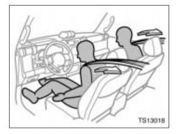
The driver and front passenger seat belt pretensioners are designed to be activated in response to a severe frontal impact.
