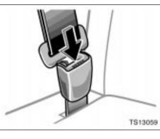
2. To remove the booster seat, press the buckle release button and allow the belt to retract.
