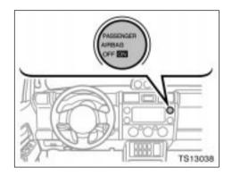
The front passenger occupant classification indicator light indicates the actuation of the front passenger airbag, side airbag on the front passenger seat.
