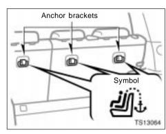
Use the anchor brackets behind the rear seatbacks to attach the top strap.
