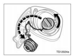
2. To remove the fuel tank cap, turn the cap slowly counterclockwise, then pause slightly before removing it. After removing the cap, hang the tether as shown in the illustration.
