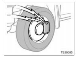
The brake pad wear limit indicators on your disc brakes give a warning noise when the brake pads are worn to where replacement is required.
