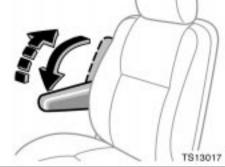
To adjust the armrest, lower the armrest to the lowest position and raise it to the desired angle. Raising the armrest to the highest position unlocks the armrest to let you return it to the lowest position.
