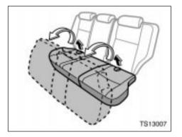
1. Swing the bottom cushion up by pulling the lock release strap.
