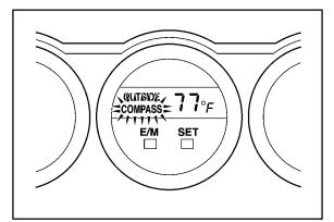
2. Switch the mode to the Compass Correction mode by pushing the "SET" button for about 2 seconds until the zone number appears on the outside temperature display.
