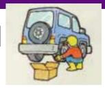
but makes correction easier. If the vehicle gets stuck, the chains can be removed and reattached to the front tires for traction. Where chains should be attached (front or rear tires) is a case-by-case decision, but generally it is recommended to use the rear tires
