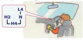
As a general rule, shifting into 4WD is to be done while the car is parked. Yet, there are types of 4WD that allow the shifting to be done while the vehicle is in motion. Confirm the appropriate procedure (by consulting the operation manual) so as not to damage the vehicle and to avoid accidents. When the shift is made, usually an indicator lamp lights up to confirm the shift. However, the lamp can fail and driving the car is a better way of confirming that the shift into 4WD has taken place.
