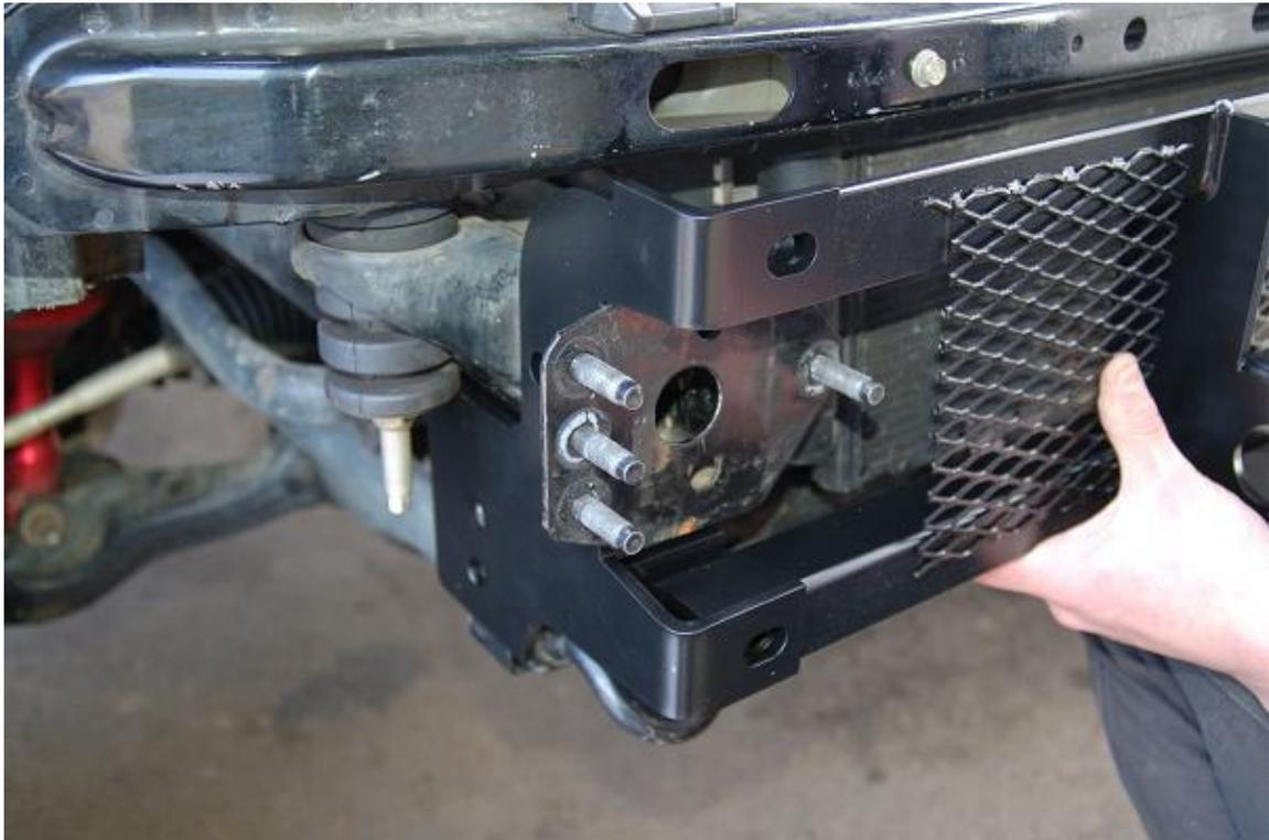
15. **[TOOL: 17mm socket, 3/4" socket, 3/4" box end wrench]** Install the passenger side plate upper 1/2" x 1 1/2" bolt with, two washers and one lock washer. Repeat the steps used for the drivers side. Keep the plate losses for now.
