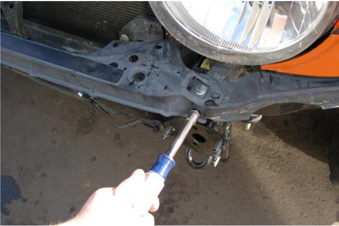
5. **[TOOL: Drill with 1/2" drill bit]** Drill out the small threaded hole on the outside of the frame directly behind each front bumper flange. Dill out only the one side of the frame. See photo:
