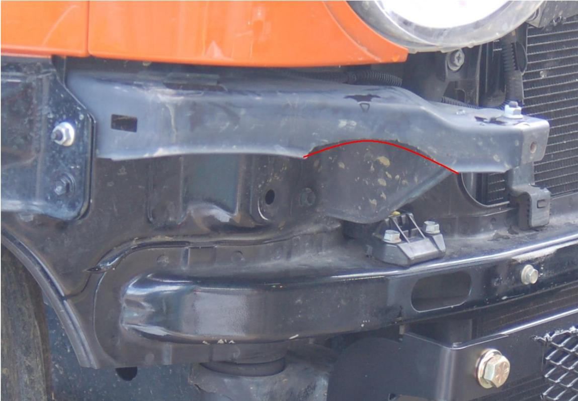
20. [TOOL: 14mm deep socket] Install the tube bumper on the front frame flanges. Tighten each of the factory 14mm flange nuts. See photo:
