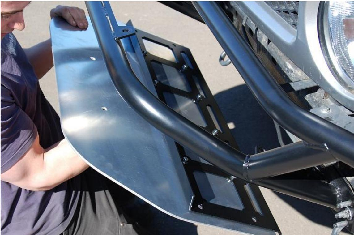
7. Using the provided four 3/8" x 2.5" stainless steel button head bolts, eight washers and four nylock nuts, bolt the bash plate in place with the provided tube spacer between the bash plate mid brace and the inner face of the mounting tabs on the tube bumper.
