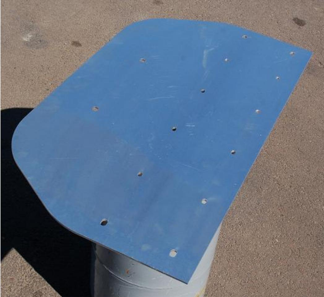
2. Set the back side support on the main bash plate. Make sure the bent edge that is 90° is facing up and the 30° edge is facing down over the edge of the bash plate. See photo:
