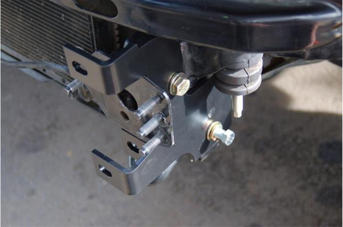
10. [TOOL: 3/4" socket, 3/4" box end wrench] Install a 1/2" washer and 1/2" lock washer inside the frame on the 1/2" bolt you just installed. Tip: To hold and thread the 1/2" nut using the 3/4" box end wrench, put a small piece of packing tape over one side of the box end wrench. See photo:
