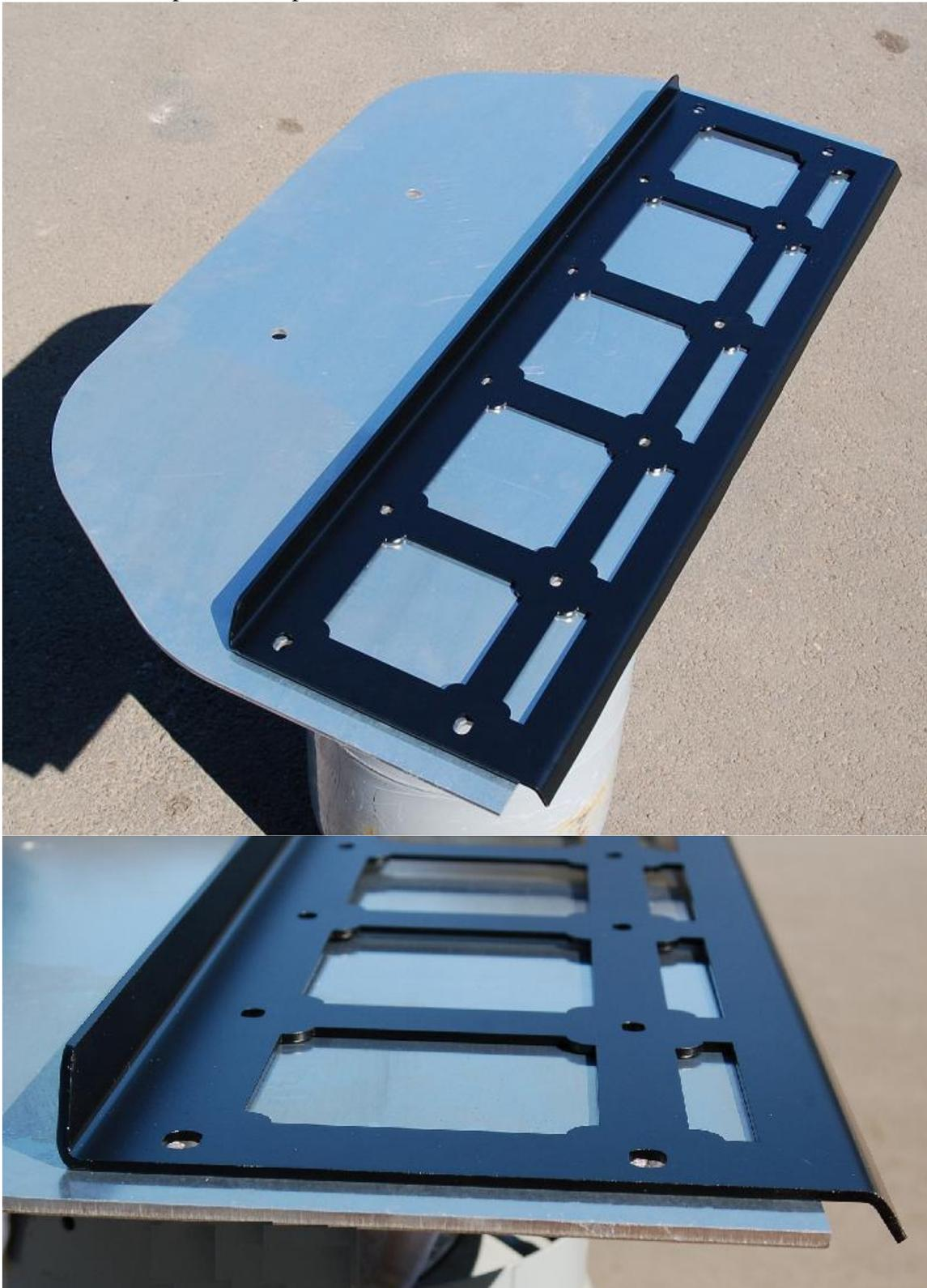
3. Use the 8 provided 1/4" stainless steel button head bolts, 16 washers and 8 nylock nuts bolt the 8 center slots together. NOTE: Put the button heads of the bolts on the opposite side of the main bash plate from the brace. This way the bolt heads face out to the front of your truck.
