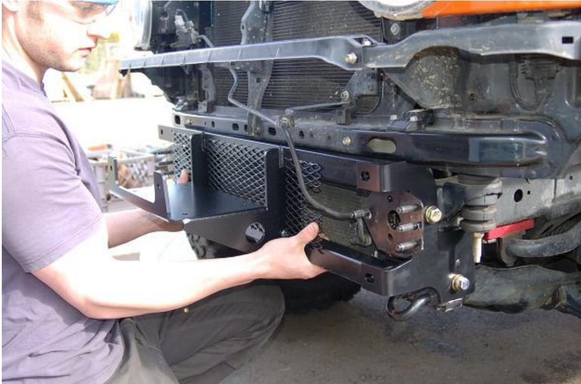
14. **[TOOL: 17mm socket, 3/4" socket, 3/4" box end wrench]** Install the passenger side, winch side plate. Once the plate is on the side of the frame the 1/2" dowel pin will hold the plate in place. Install winch mount lower 1/2" x 3" bolt to hold the winch beam in place. See photo:
