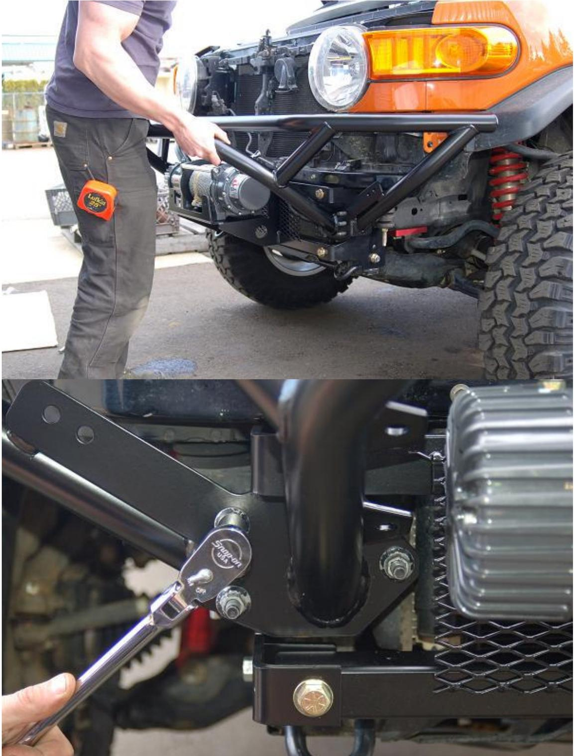
21. Use the supplied flange bracket to install the winch controller box on the bumper.
