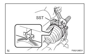
(e) Using SST, measure the clearance of the boot clamp as shown in the illustration.
