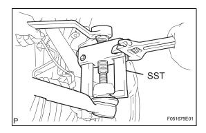
(b) Using SST, separate the tie rod end from the steering knuckle.
