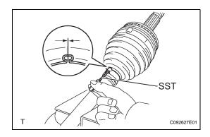
(d) Using SST, measure the clearance of the boot clamp as shown in the illustration.
