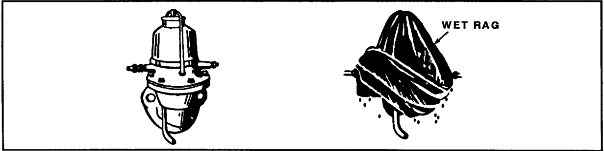
FIGURE 22-18. Fuel Pump Vapor Lock Correction.
